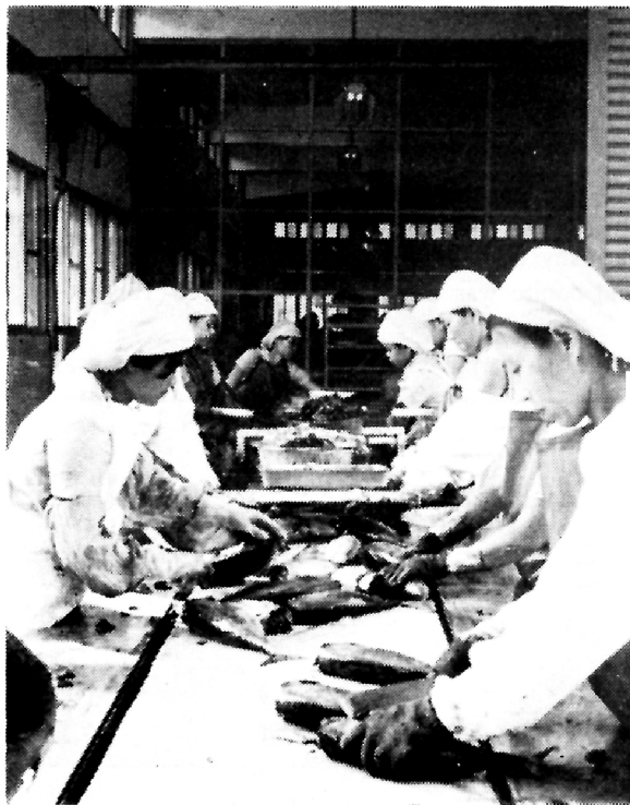
Fig. 4-3. Bonito being eviscerated on the butchering table (in the middle of which runs a slow-moving belt conveyor).
