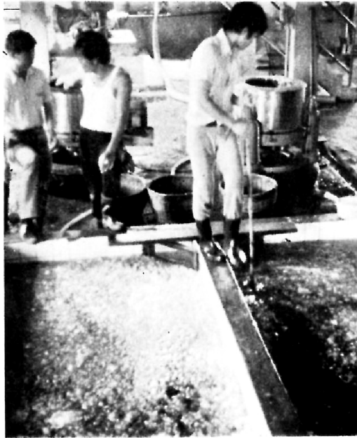
Fig. 7-9. Washing the Melted Pieces of Agar After Bleaching.
